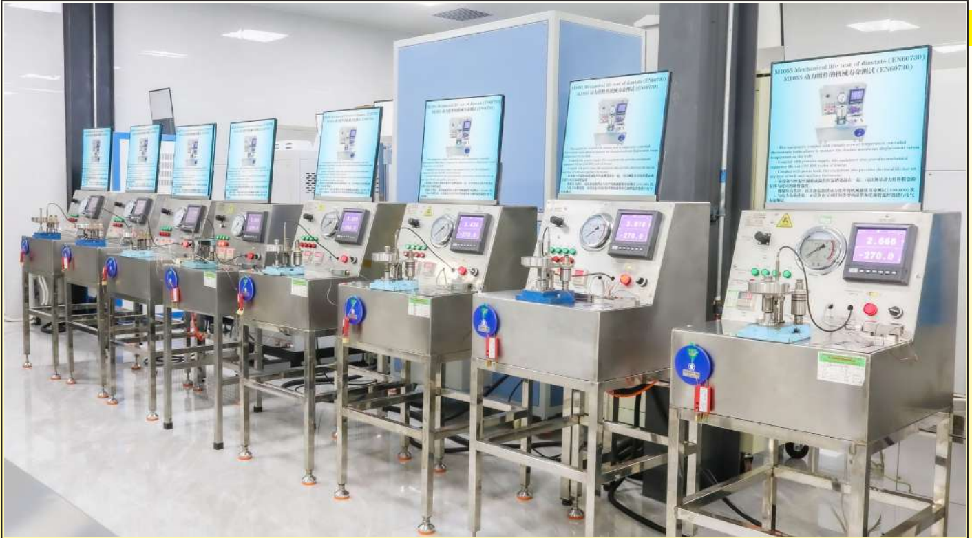
Set of diastats mechanical life test automatic equipment. Each equipment is equipped with a data recorder of testing parameters and number of cycles. (Ultimheat laboratory).
